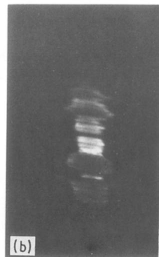
Figure 10 (a) Irregular stacking of SiC lamellae for AC1 SiC whiskers with (b) axial dark field. (d-spacing diffraction disk = 0.24 nm).
